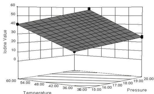
Figure 4. Response surface plot of iodine value as a function of temperature and pressure
