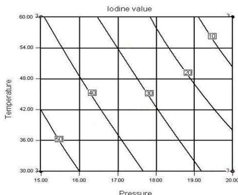
Figure 5. Contour plots of iodine value as a function of temperature and pressure
